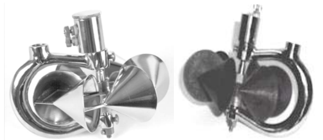
Рис. 10. Вертушка Прайса USGS TYPE AA-ICE MODEL 6240, USGS TYPE AA-ICE-P MODEL 6245 (Rickly Hydrological Company, США) (по [12; 19])
